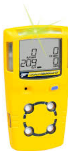
Photo 2-2. Typical Personal Four-Gas Monitor
